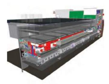
Sectional view of Titiwangsa Station reflecting system and MEP services arrangement for a two-level station
